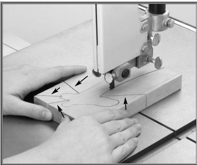
Figure 52. Relief cuts before cutting curves.
